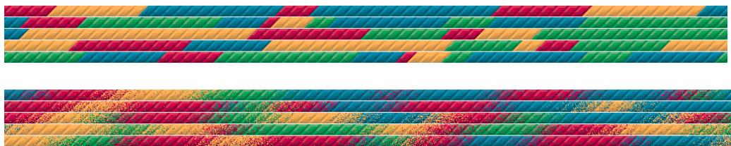
Figure 215: Multicolor yarn without smooth (top), and with the smooth option set to 15
