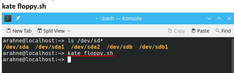
Figure 427: Opening the `Kate` text editor and creating a file in a single-line command
