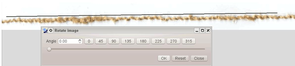
Figure 227: Aligning a yarn after scanning
