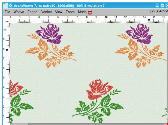
Figure 289: Simulation with two extra wefts in four colors
