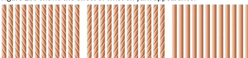
Figure 206: Yarn with twist sense S, Z, and without twist
