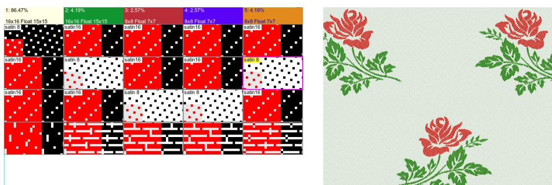
Figure 290: Same jacquard conversion as on Figure 288 but without yarn letters produces fabric with only two colors in extra weft.
