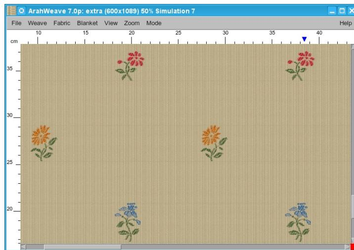
Figure 169: Extra weft fabric with solid ground weft
