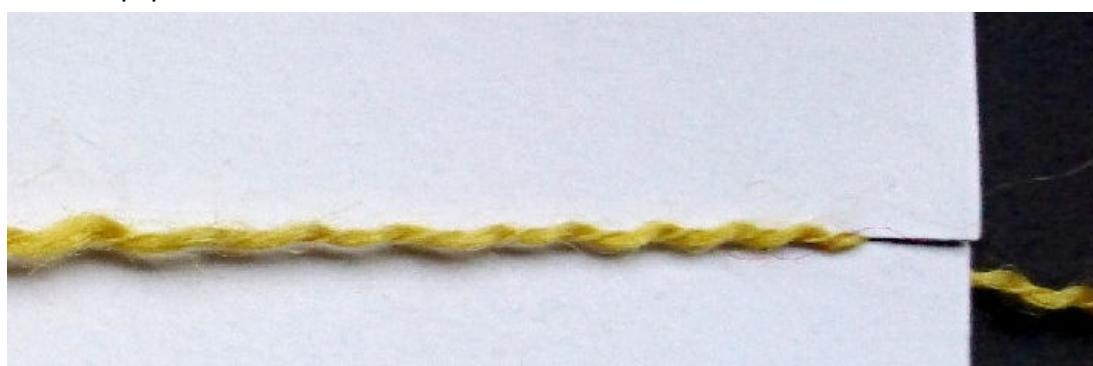
Figure 226: To prepare a yarn for scanning, cut a notch at each side of a paperboard, and anchor a thread in the notches.
