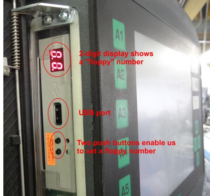
Figure 400: USB floppy emulator installed on Stäubli JC5 controller
